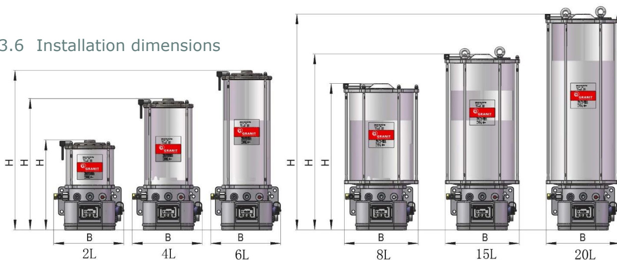
Fig. 11.1 Installation dimensions of the ALPB pump reservoir, 2-6 litres D170mm, 8 to 20 litres D230mm
