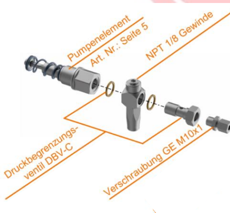
Fig. 16.2 Exploded view PE with PRV-C
