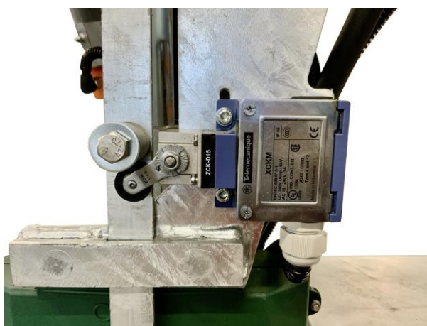
Fig. 6. Limit sensor for the closed position of the suction channel latch
