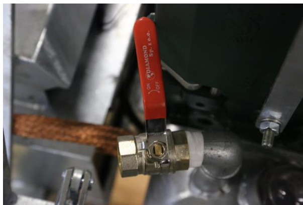
Fig. 41. Vent valve in closed position
