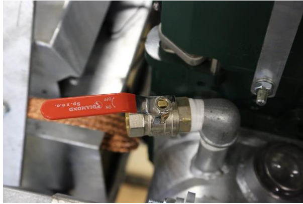
Fig. 40. Vent valve in open position
