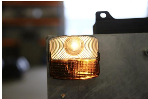
Fig. 39. Signalling of the opened suction channel latch and closed return channel latch
