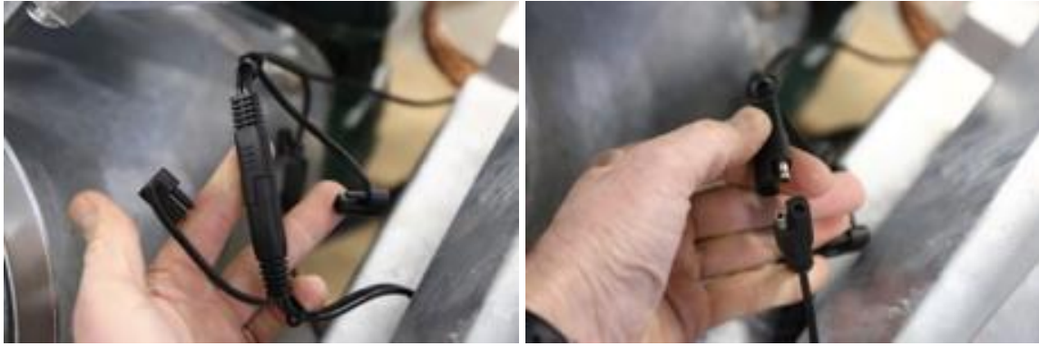
Fig. 9. Double banana plug-socket arrangement, wires from the output side of the charger to the battery - view of connected and disconnected elements
