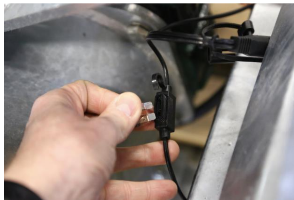
Fig. 10. A 7.5 A car-type plate fuse on the output side of the battery charger
