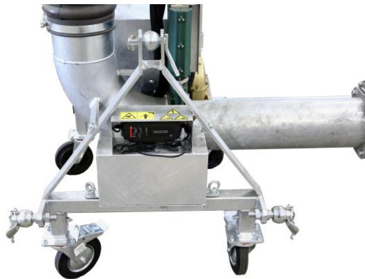
Fig. 32. Three-point hitch system for the front and rear three-point linkage at the tractor
