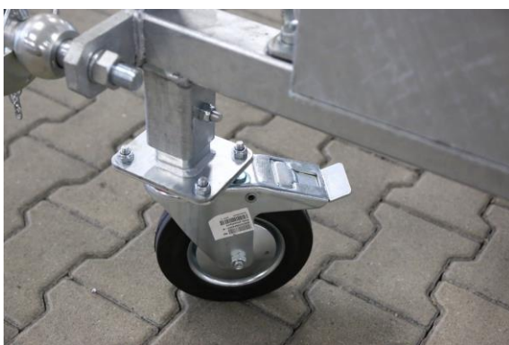
a) brake not locked
