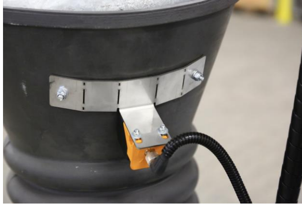
Fig. 5. A sensor detecting the steel tip nozzle of the water or slurry tanker in the funnel docking station
