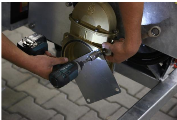
Fig. 18. Plug disassembly from the return channel opening - disassembly view using a flat wrench, a socket wrench and a screwdriver
