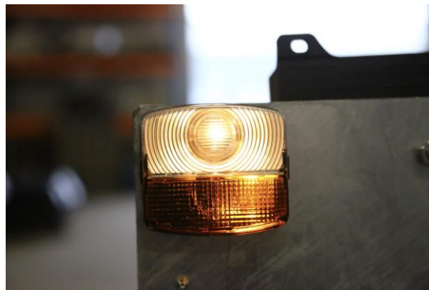
Fig. 28. Signal lamp - view with the white and orange lights on
