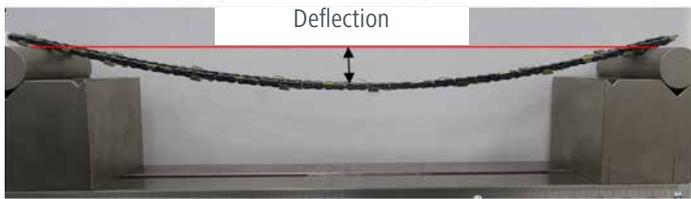
Image 1: Test setup for measuring saw chain deflection
